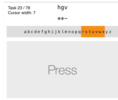
Figure 2. The Wizard of Oz keyboard with cursor width as 7, used to collect users' typing data
