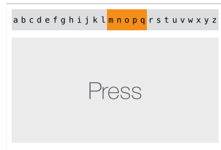
Figure 1. The experiment interface in the pilot study. Only the alphabetical layout and a 5-letter-wide cursor are presented. The orange window is the sliding cursor to select letters, whose position is depended on the pressure level.
