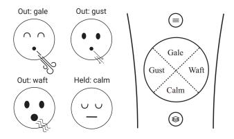
Figure 1: Left: The four breathing actions. Right: Actions mapped to four areas on the HTC Vive controller trackpad.
