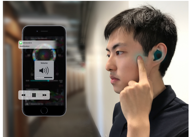
Figure 1: EarBuddy leverages the microphone embedded in wireless earbuds to recognize gestures on the face or around the ears.
