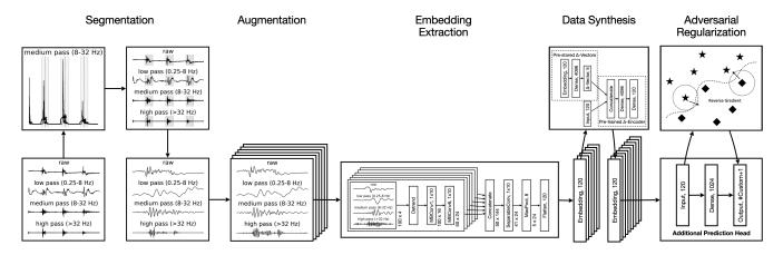
Figure 5: The Data Processing Pipeline of Training a Gesture Customization Prediction Head. It starts with a short data sequence (3 shots in this example) recorded by an end-user and goes through data segmentation, augmentation, and synthesis before the training. The training process is enhanced by adversarial regularization.
